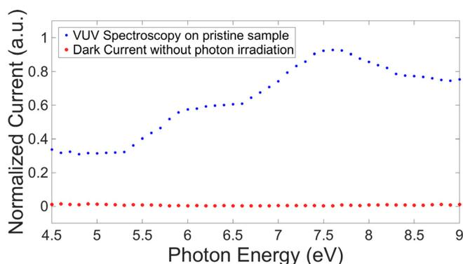
FIG. 1. Comparison of VUV photoemission spectroscopic measurements on 150 nm SiCOH and normalized dark current.
