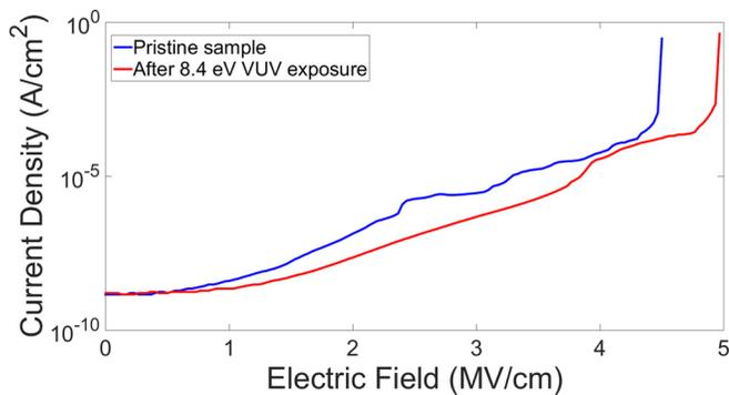
FIG. 3. Comparison of I-V characteristics of 150 nm SiCOH test samples before and after 8.4 eV VUV irradiation with  $1.3 \times 10^{14}$  photons/cm<sup>2</sup> fluence.
