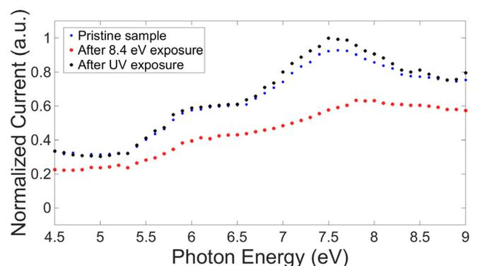
FIG. 4. Comparison of VUV photoemission spectroscopic measurements of pristine SiCOH samples and samples after 8.4 and 4.9 eV photon irradiation.
