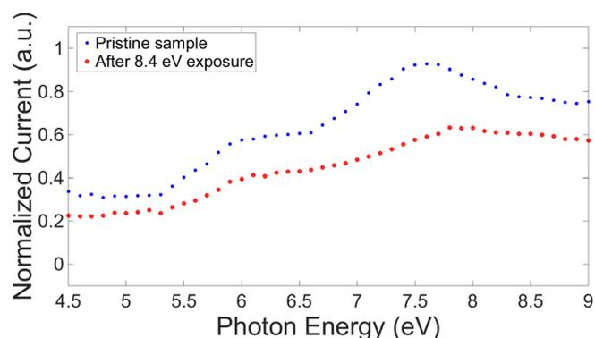
FIG. 2. VUV photoemission spectroscopic measurements on 150 nm SiCOH before and after 8.4 eV VUV irradiation with  $1.3 \times 10^{14}$  photons/ $\text{cm}^2$  fluence.
