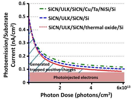
Fig. 2. Photoemission flux of SiCN/SiCOH/SiCN deposited on Cu, Si and Si with thermal oxide as a function of increasing dose of 8-eV VUV photons.
