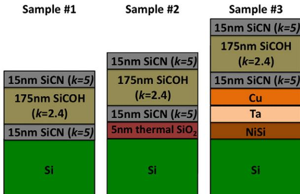
Fig. 1. The dielectric stack of SiCN/SiCOH/SiCN deposited on three different substrates.
