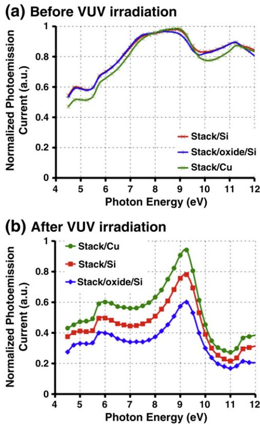
Fig. 3. VUV spectroscopy at 4.5–12 eV for SiCN/SiCOH/SiCN deposited on Cu, Si and Si with thermal oxide (a) before 8-eV VUV irradiation and (b) after 8-eV VUV irradiation.
